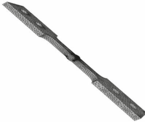
Figure 4. Detail of the mesh generation for the weld joint model.
