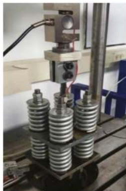
Figure 2. Specimen mounted on the uniaxial fatigue machine.
