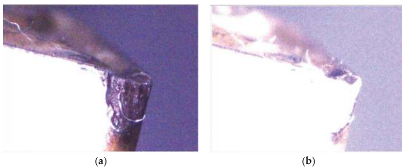
Figure 4. Captured flank and insert exposure images. (a) Flank exposure image; (b) Insert exposure image.
