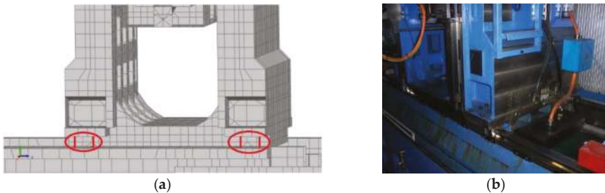
Figure 4. Connections between bed frame and column in a (a) FE model and (b) photograph.
