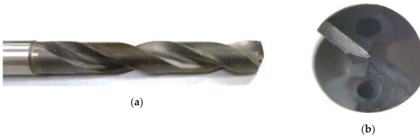
Figure 1. The diamond-coated carbide drill bit with a 7.6 mm diameter that were tested. (a) Lateral view. (b) Frontal view.
