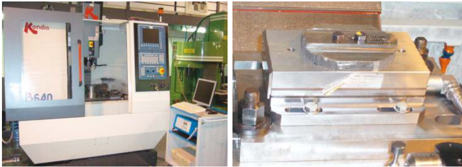
Figure 1. Kondia ® model B640 (left) and Kistler ® 9257B dynamometer (right).
