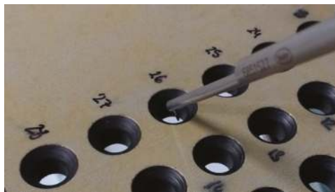
Figure 2. Hole profile and roughness analysis of a carbon fiber reinforced plastics (CFRP) coupon with a contact profilometer.
