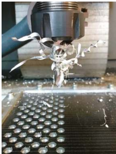
Figure 8. Adhesive and aluminium alloy chips adhered to the cutting geometry.
