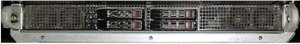
Figure 1. The HPC solution for the ICARUS project is based on the Server Supermicro RTG-RZ-1240I-NVK2 (source: ICARUS).
