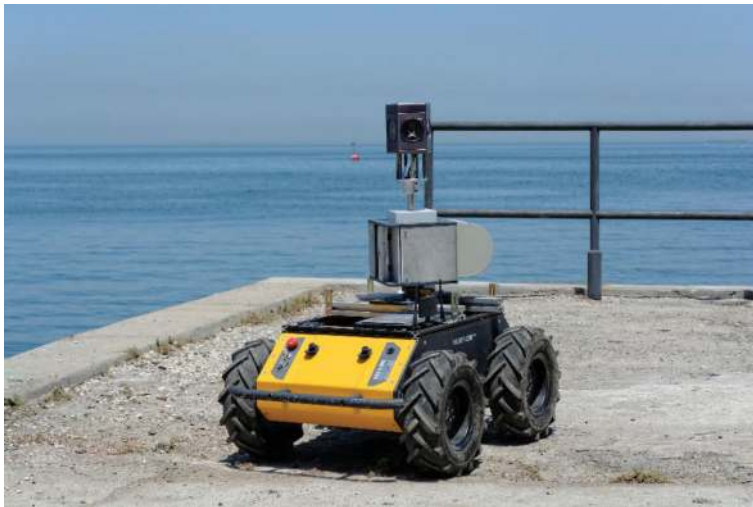
Figure 10. Dedicated support system—mobile mapping platform (source: ICARUS).
