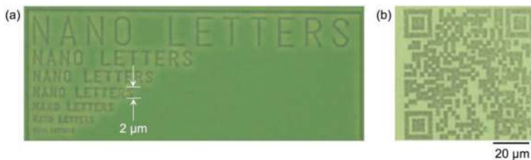
Figure 12. (a) Optical microscope image of the plasmonic text (“NANO LETTERS” with different sizes) realized by the DLW technique. (b) Optical image of a quick response (QR) code, which links to the website of the author’s laboratory (LPQM).
