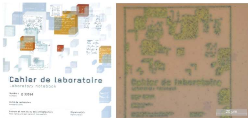
Figure 13. The color printed image fabricated by the DLW method on Au film. Left: a real "experiment book". Right: a plasmonic image of corresponding book at microscale.
