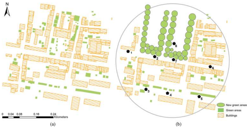
Figure 2. Computational domain for (a) the baseline scenario and (b) the green scenario, including the wind speed measurement point location, or the corresponding computational cells in the CFD simulations. The newly implemented green areas are represented by green circles.
