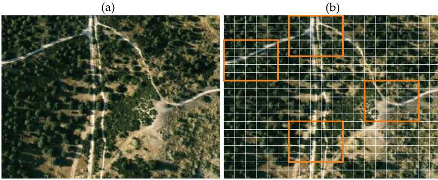
Figure 8. (a) Example of a real environment modelled as a grid map. (b) Patches of terrain used for training are marked with an orange box.
