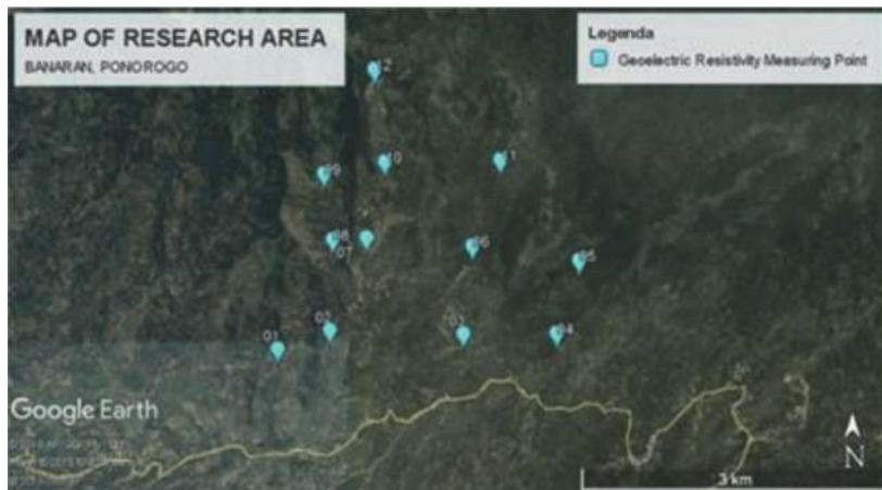
Figure 5. Distribution of geo-electric resistivity measurement points.
