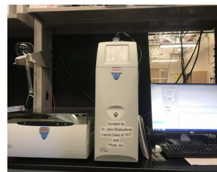
Figure 2a: IC set up used to analyze the anions from the water samples and the diluted standard series.
