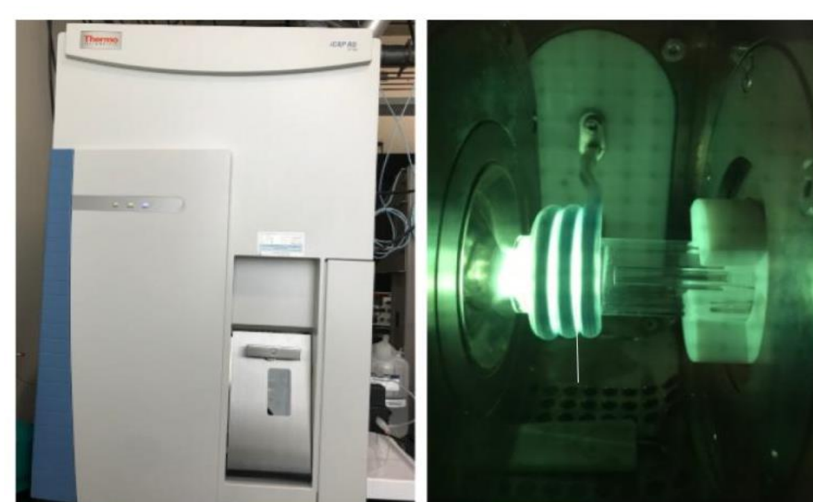
Figure 3a: ICP-MS and the speciation column inside the system that ionizes the samples, produces flames and atomizes the sample for detection.
