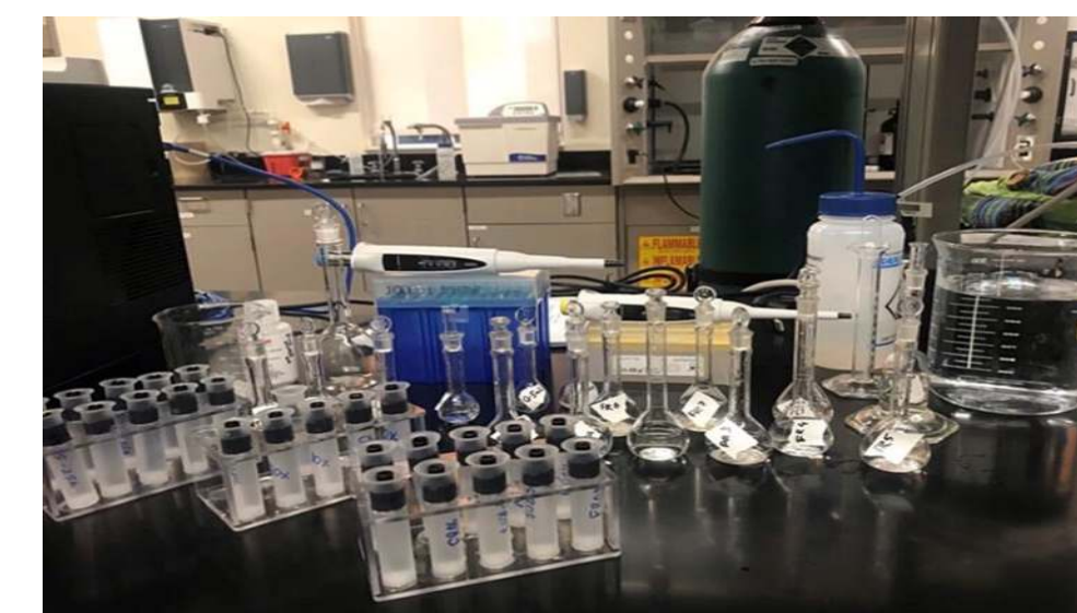
Figure 2b: Set of samples prepared in the conical flasks and 10 mL of it transferred in polyvials to analyze anions present in them.
