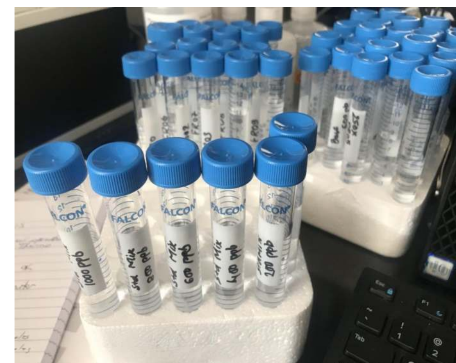
Figure 3b: 10 mL of standard, diluted water samples from the sites and diluted water samples in 15 mL falcon tubes ready for analysis in ICP-MS.
