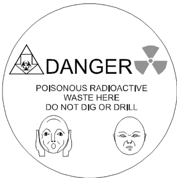
Figure 4. Permanent Marker Warning Sign.
