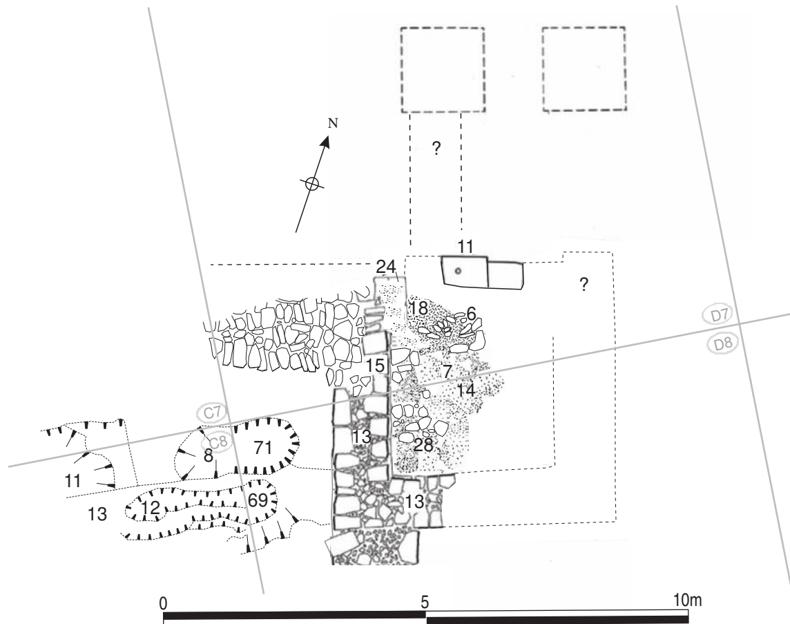
Figure 17.11: West Gate, south guardchamber, latest surface (late third/early fourth century?) at 1:100.
