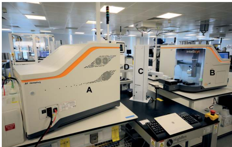
Figure 8. Automation platform used with our iQue ® Screener HD. (A) and (B) iQue ® Screener HD, (C) ACell robotic arm, (D) NanoServe ™ stacker carousel.
