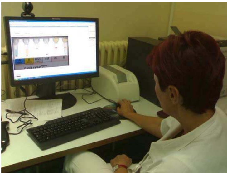
Fig. 3. Laboratory setup of the telemedical system. Main application window can be observed on the terminal. Gelscope device is visible right next to the terminal monitor. Videoconference call is not established.
