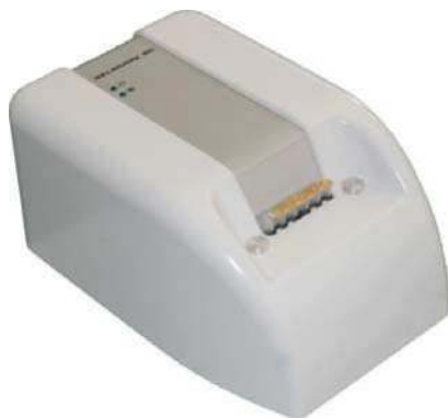
Fig. 7. Special purpose hardware for capture of gel-card images, Gelscope 80 - version 2.
