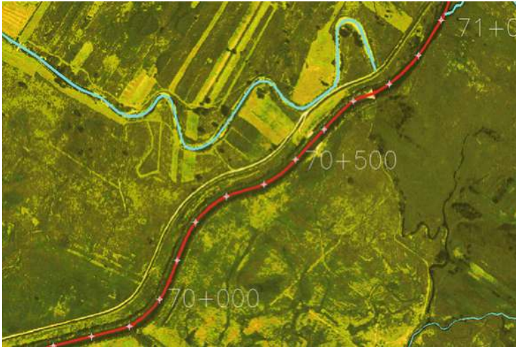
Fig. 5.7 The curvature comparison of the natural ( blue ) and regulated ( red ) river channel
