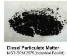
Figure 1: Standard Reference Material (SRM 2975) of Diesel Particulate Matter, from an industrial forklift.
