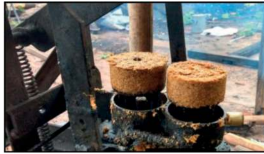
Figure 10. “BR 1” rice husk briquette prototype 1.
