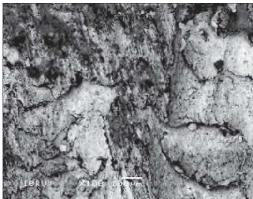
Fig. 5. SEM Image of Wear Tested Pure Cu sample
