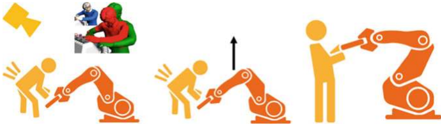
Fig. 2 Concept of the WPC. An actuator, in this case a robot, holds the workpiece to be processed. Additionally, a sensor system monitors the worker’s posture. In case the posture becomes physically straining, the WPC proposes the change to the workpiece pose, making it possible for the user to adopt a more natural posture
