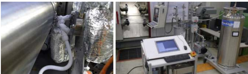
Fig. 10 Internally-cooled turning tool and cooling periphery
