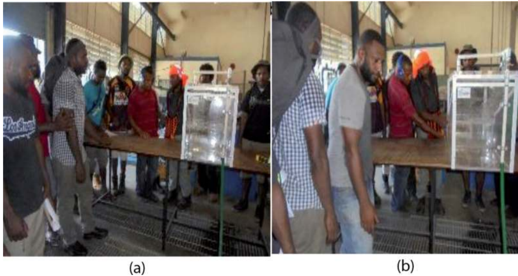
Figure 8. (a) Test on water tightness of tanks; (b) demonstration of rainwater simulating falling to the catchment area of RHI model.
