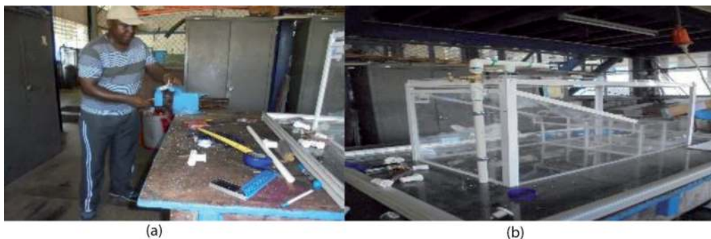
Figure 7. (a) RHI model piping system on the making by Carl Smith; (b) the rainwater simulator represented by showerhead system placed at a distance from a rain tray, surface runoff, and the storage tank of RHI model.
