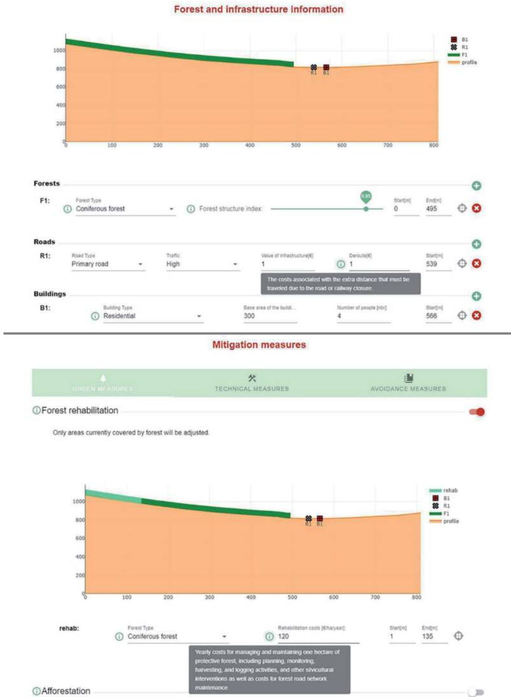
Figure 10. Protective Forest Assessment Tool (FAT) web interface. Upper panel: information about the existing forest, buildings, and roads to be protected need to be entered by the FAT user. Lower panel: green, technical, and avoidance mitigation measures can be selected via dropdown menus. Info buttons guide the user through each step.
