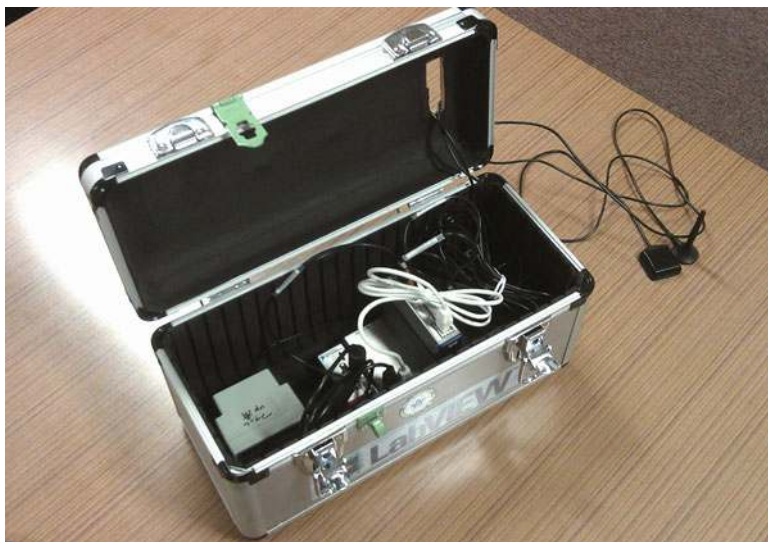
Fig. 10.4 The in-vehicle unit of KURAMA-II. A CsI detector and a CompactRIO are compactly placed in a toolbox with the size of 34.5 \times 17.5 \times 19.5 cm
