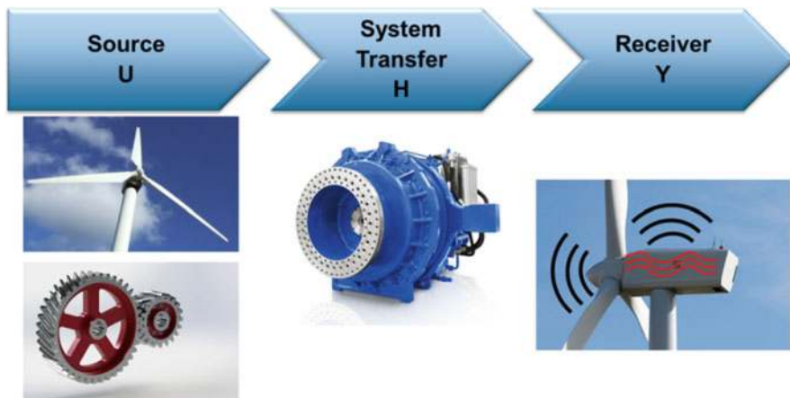
Fig. 10.1 The Source-Transfer-Receiver approach applied to a wind turbine gearbox
