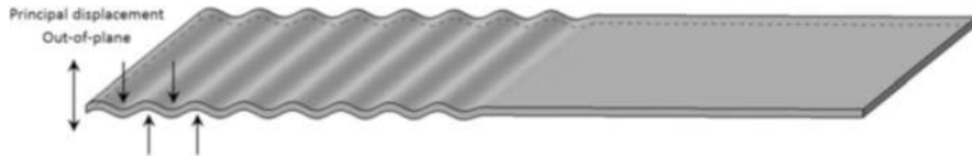
Fig. 3.9 Antisymmetric mode of propagation
