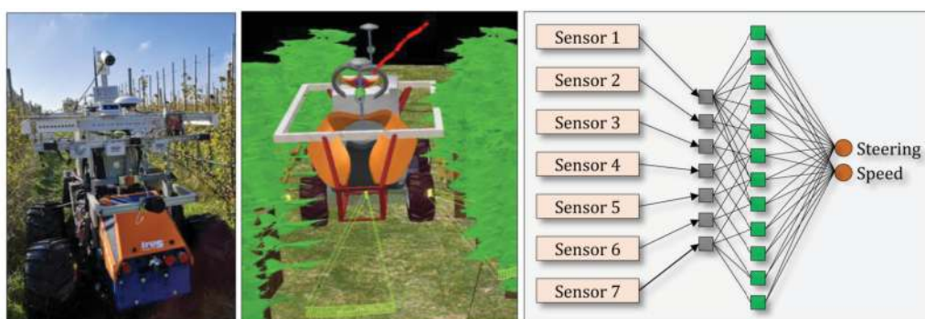
Figure 11. Application of machine learning as a knowledge-based control approach for assisted navigation of a four-wheel steering field robot agent. Source: SunBot.de.
