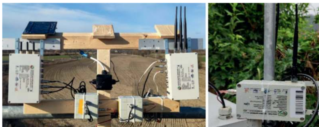
Figure 14. Redundant LoRa sensors with modular accessories and multiple transmitters and gateways to overcome uncertainties and connectivity issues in actual field conditions. Source: SunBot.de.
