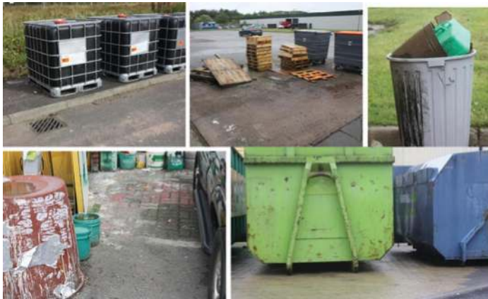
Figure 17.12 Uncontrolled waste storage on industrial yards, contrasted with waste storage units on a modern industrial estate: sealed containers, with no exposure to rainfall, and no drainage outlets.
