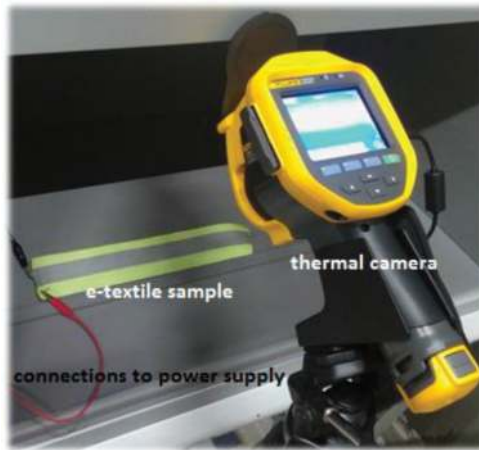
Figure 10. Testing set up to measure surface temperature.
