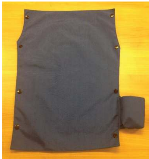
Figure 13. E-textile-based thermal heating panel to be placed inside the heating vest.
