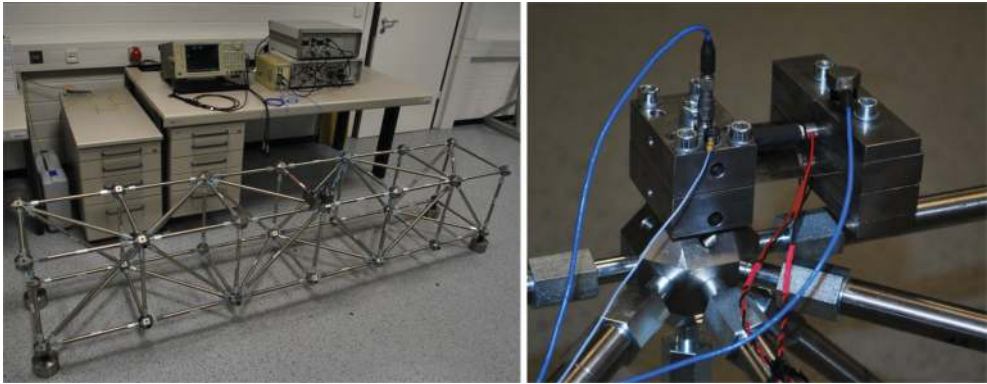
Figure 16. Test setup for the active control experiment (left) and detail of the actuator instrumentation (right).
