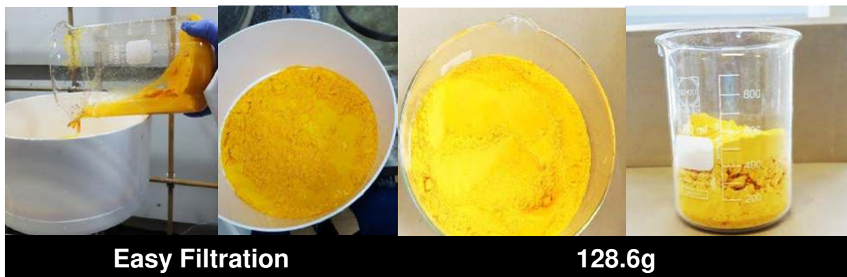
Figure 6. Scale-up for COP-222 synthesis with terephthalaldehyde (200g) and ammonium chloride (320g) in dimethylformamide (1.5L)
