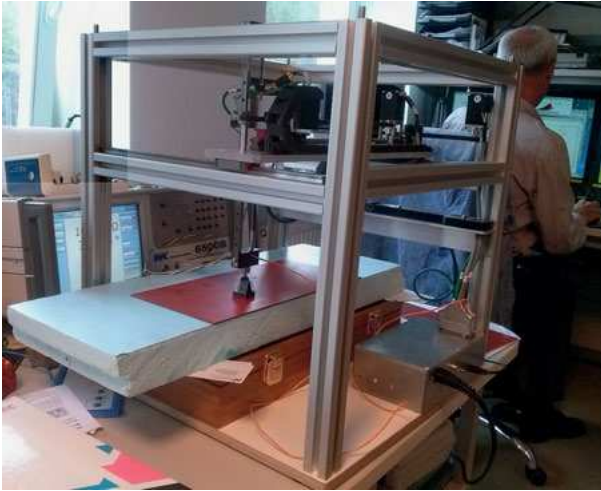
Fig. 3: Developed eddy current scanner.
