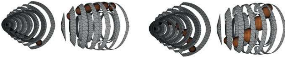
Fig. 7: Electrode positions 1 and 2 with sensitivity spaces (spheres).
