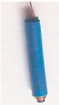
Fig. 10: Sensor coil with ferrite core.
