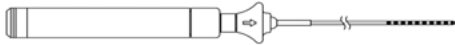
Fig. 3: Catheter that is inserted into the right ventricle through the pulmonary artery to measure impedance change (INQUIRY™ electrophysiology catheter).
