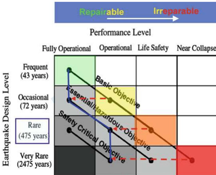
Fig. 13.5 Seismic Performance Design Objective Matrix as defined by SEAOC Vision 2000 PBSE Guidelines, herein rearranged to match building tagging, and proposed/required modification of the Basic-Objective curve towards a damage-control approach (blue line, Modified after Pampanin (2010), Kam et al. (2011))
