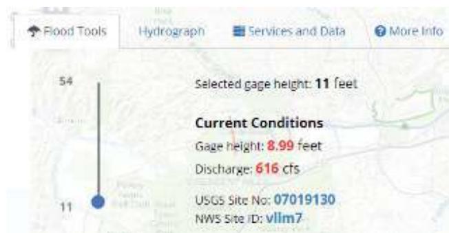
Figure 4. FIM sliding gauge height tool.
