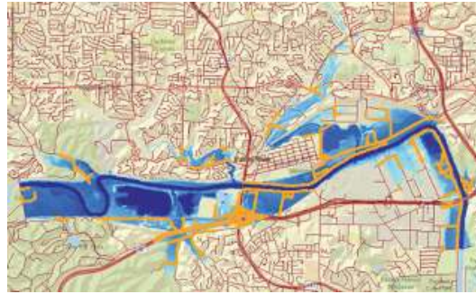
Figure 12. Flood affected road segments for flood inundation profile corresponding to 45 ft. stage value for Valley Park, Missouri.
