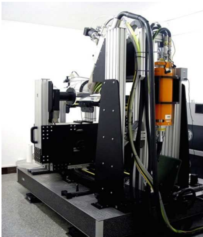
Fig. 2.6 ACTIS300-320/225 X-ray industrial CT testing system
