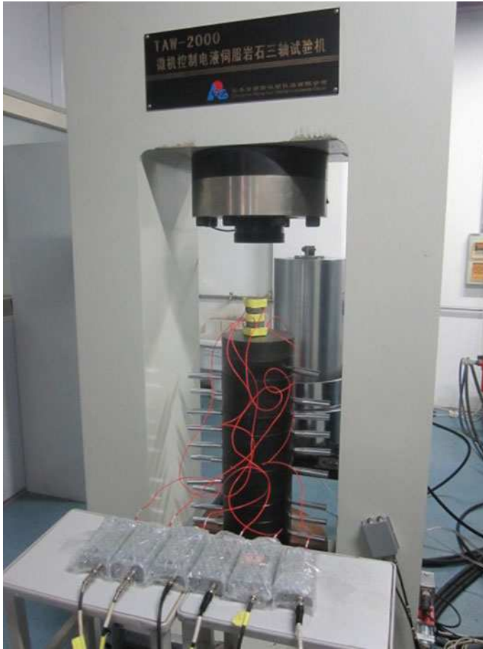
Fig. 2.3 TAW-2000 computer control electro-hydraulic servo rock triaxial testing machine
