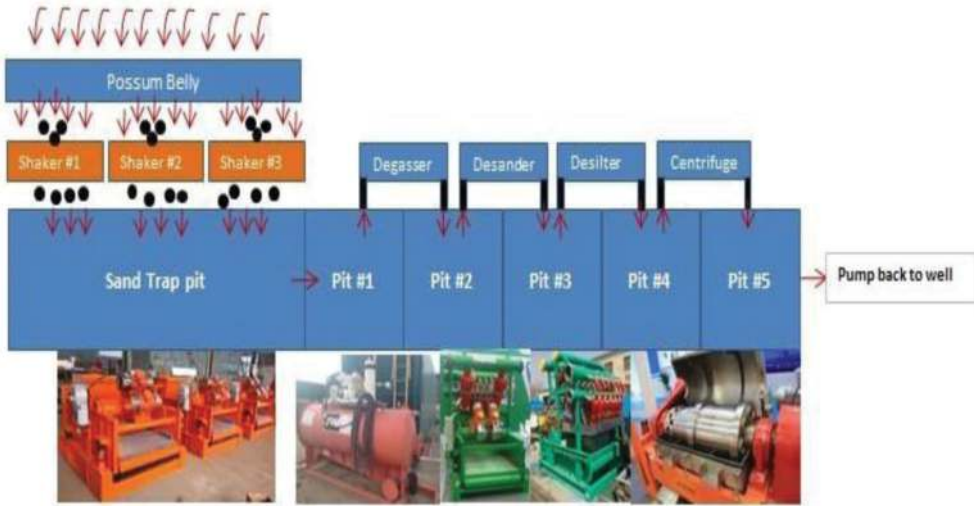
Figure 3. Old design solid control system.
