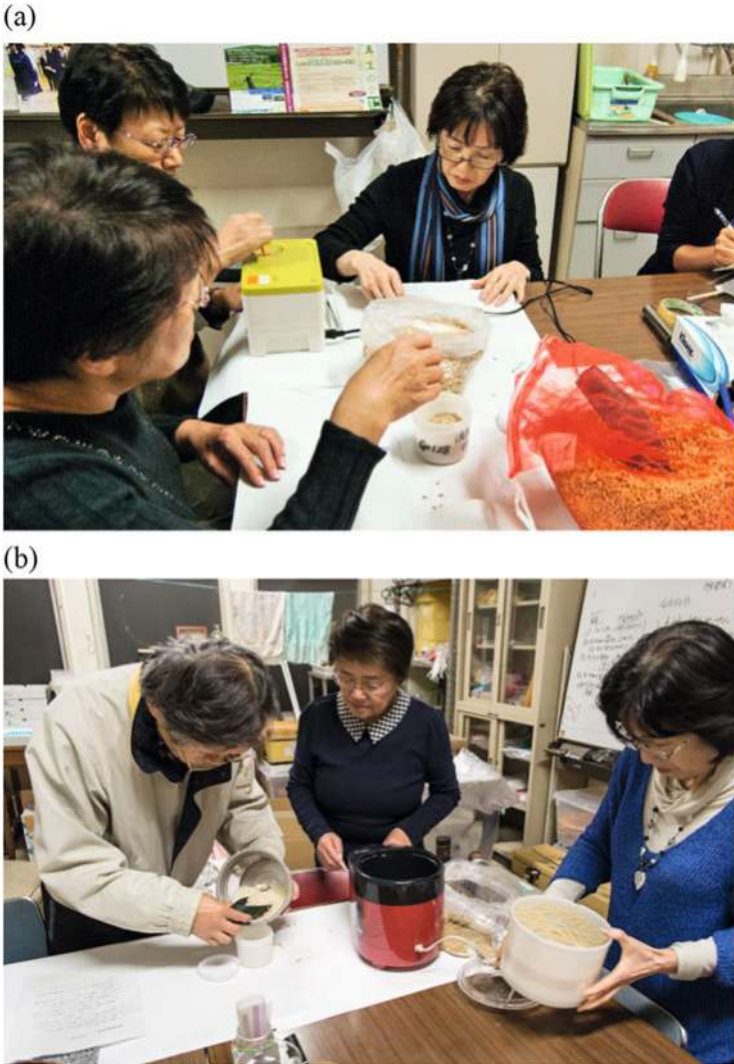
Fig. 6.6 (a) Hulling process of unhulled rice to give brown rice, being performed at “Circle Madei”. (b) Polishing process of brown rice to give white rice and rice bran, being performed at “Circle Madei”
