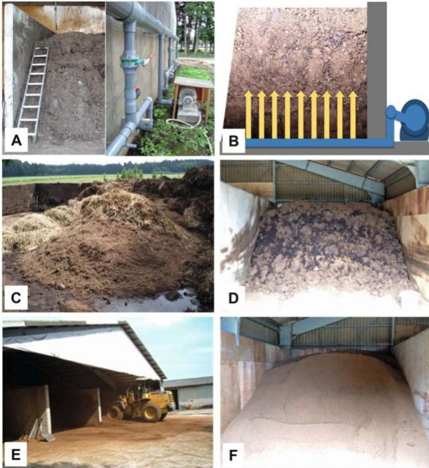
Fig. 8.1 Aerobic ultra-high temperature fermentation process for livestock feces and farm residues. (a and b) Overview of fermenters (4.3 m width \times 2.4 m height \times 8 m depth). Three side walls and a floor were made of concrete. An appropriate amount of air was supplied from 2 vinyl chloride tubes installed in the floor grooves of the floor without interruption from the electric blower, which was placed outside of the fermenter. (c) Feedstock (mixture of the excretions of farm animals, litter residues, livestock feed residues, and residues of crop silage and haylage) before fermentation. (d) Appearance of the fermenter at the start of the fermentation stage. Feedstock was mixed with an equal amount of the end products of fermentation (mostly the dormant spores and sprouts of high temperature fermentation bacteria). (e) During fermentation, all fermenting mixtures were moved into a neighboring fermenter using a wheel loader. This mixture process of fermenting substances was repeated every 7 days. (f) After being mixed 6 times, the fermenting substances became powdery (moisture content less than 35 %) 7 weeks after the start of fermentation. The fermented product at the final point was used as an organic fertilizer for crops and pasture cultivation
