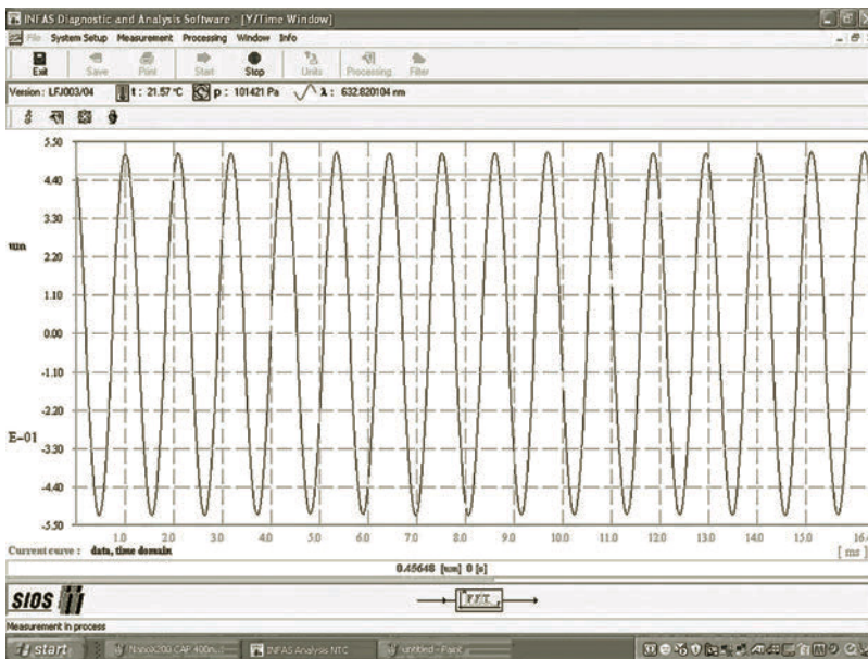
FIGURE 13.10 Demonstration of open loop repeatability of a PZT flexure.
