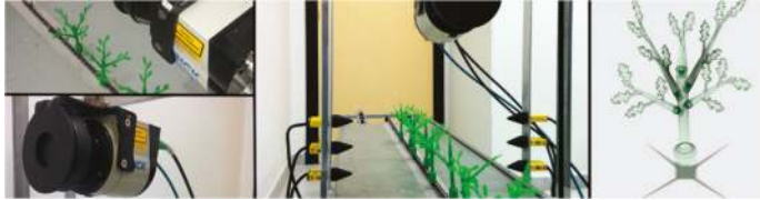
Figure 1. Details of the sensors on the laboratory platform (vertical LiDAR and Light-beam sensors) for the detection and structure of the modular 3D plant.
