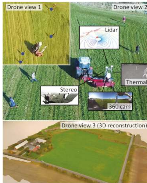
Figure 1. Recording platform surrounded by static and moving obstacles. Multiple drone views record the exact position of obstacles, while the recording platform records local sensor data.
