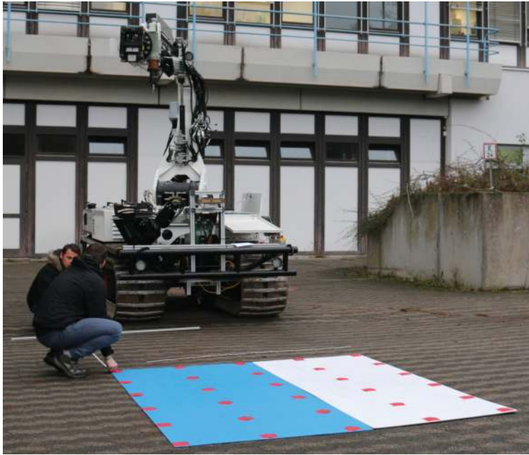
Figure 12. Calibration of the 3D vision sensor. The sensor can be seen mounted on the sensor tower of the LUGV (Source: ICARUS).
