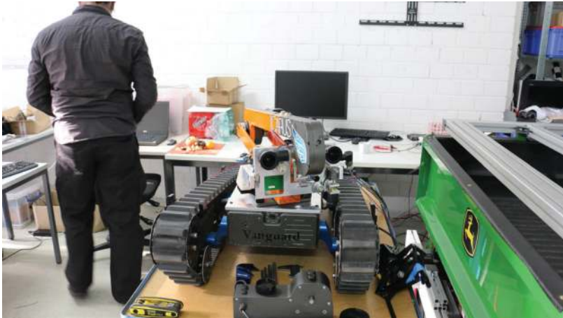
Figure 17. The SUGV with the human detection sensor mounted in front of the manipulator arm (Source: ICARUS).
