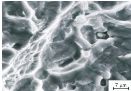
Figure 9. Fatigue fracture surfaces of Ti-6Al-5Mo-5V-1Cr-1Fe alloy cooled from 1020°C at a rate of 0.8°C s -1 .
